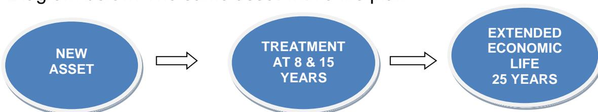
The above diagrams are simplified ways of looking at how life plans work. Carrying out economic treatments to the asset before they deteriorate to an end of life state, extending the life of that asset before it requires replacement.
